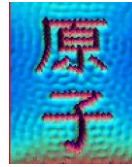
Iron atoms arranged on a copper (111) surface. These Kanji characters represent the word "atom".
